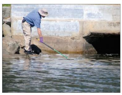
Grab samples are taken using a bottle at the end of a pole so that a sample can be taken away from the shoreline and hopefully in the flow of the water itself. This method is also used, along with the gloves, so samples are not contaminated. The city's biologists also monitor current conditions when grabbing samples at each location, to include weather, presence of people and/or animals, tidal flow, and other factors. COURTESY PHOTO | THE BEACON
